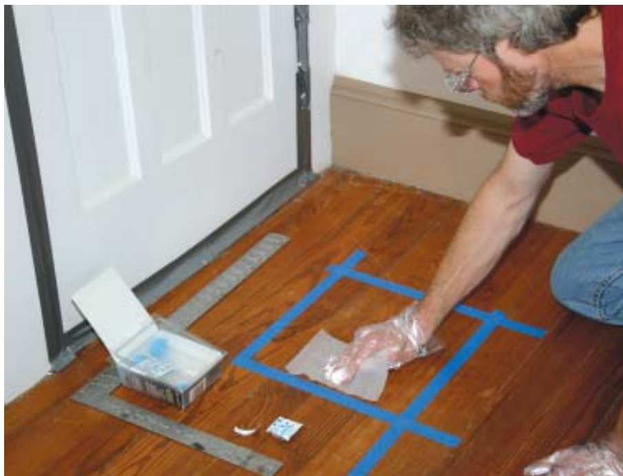
Figure 5. Swabbing a representative floor sample and sending it to a testing service (most can get you the results within 24 hours) is the way to know for sure that you've cleaned up all the lead.
